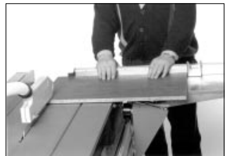
Pull sliding carriage back. Turn work around by 180°, swing flipstop down again and place squared edge against the stop. Make second cut.
